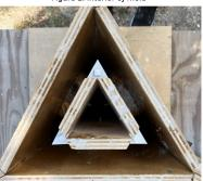
Figure 2: Top-view of assembled mold
